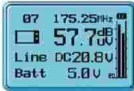
(Line AC/DC Voltage & Battery Voltage Measurement)
