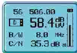
(Digital Channel Power & C/N Measurement)
